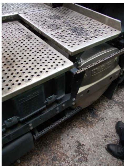
Access to 5 th wheel area of vehicle, thin bars rather than full treads makes access more difficult and may encourage drivers to jump down
